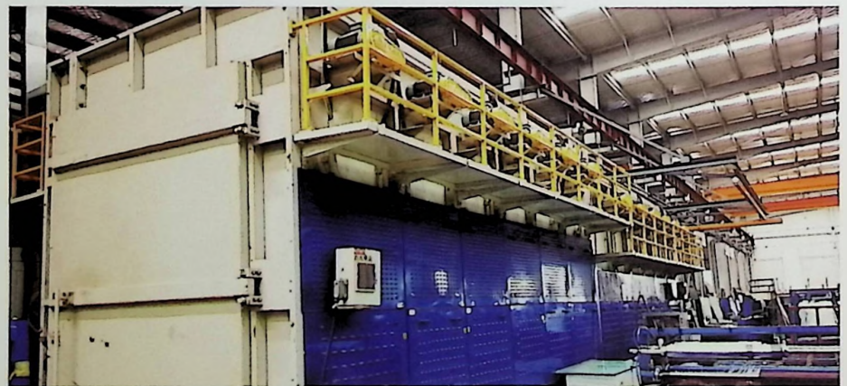
Heat Soaked Glass Furnace
