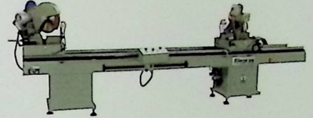
SJT02-350 塑料型材中挺切割锯 PVC win-door mid-mullion cutting saw
