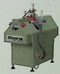
SCXZ2-60×120×3000 塑料型材双头水槽铣床 PVC Profile 2-head Auto Water-slot Milling Machine
