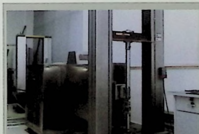
隔热型材抗剪切性能测试 thermal barrier strips anti-shearing property testing
